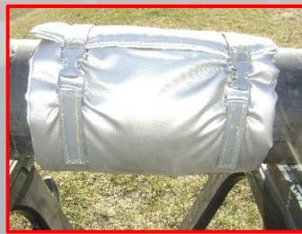
Our preheat (1,000°F fabric) and our post weld heat treat (PWHT) blankets (2,000°F fabric) are reusable and can be used up to 50 thermal cycles with one blanket. We can also design these blankets with or without tabs.
