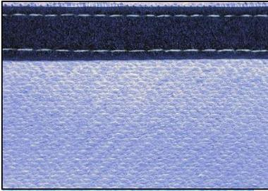
2mm Thick Coated Fiberglass Fabric on One Side
